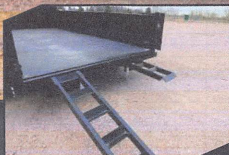
Ladder-style ramps for loading equipment, stored under dump body.
