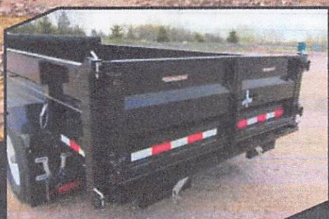
Three-way double doors open to the side, down from the top, or swing open from the bottom.
