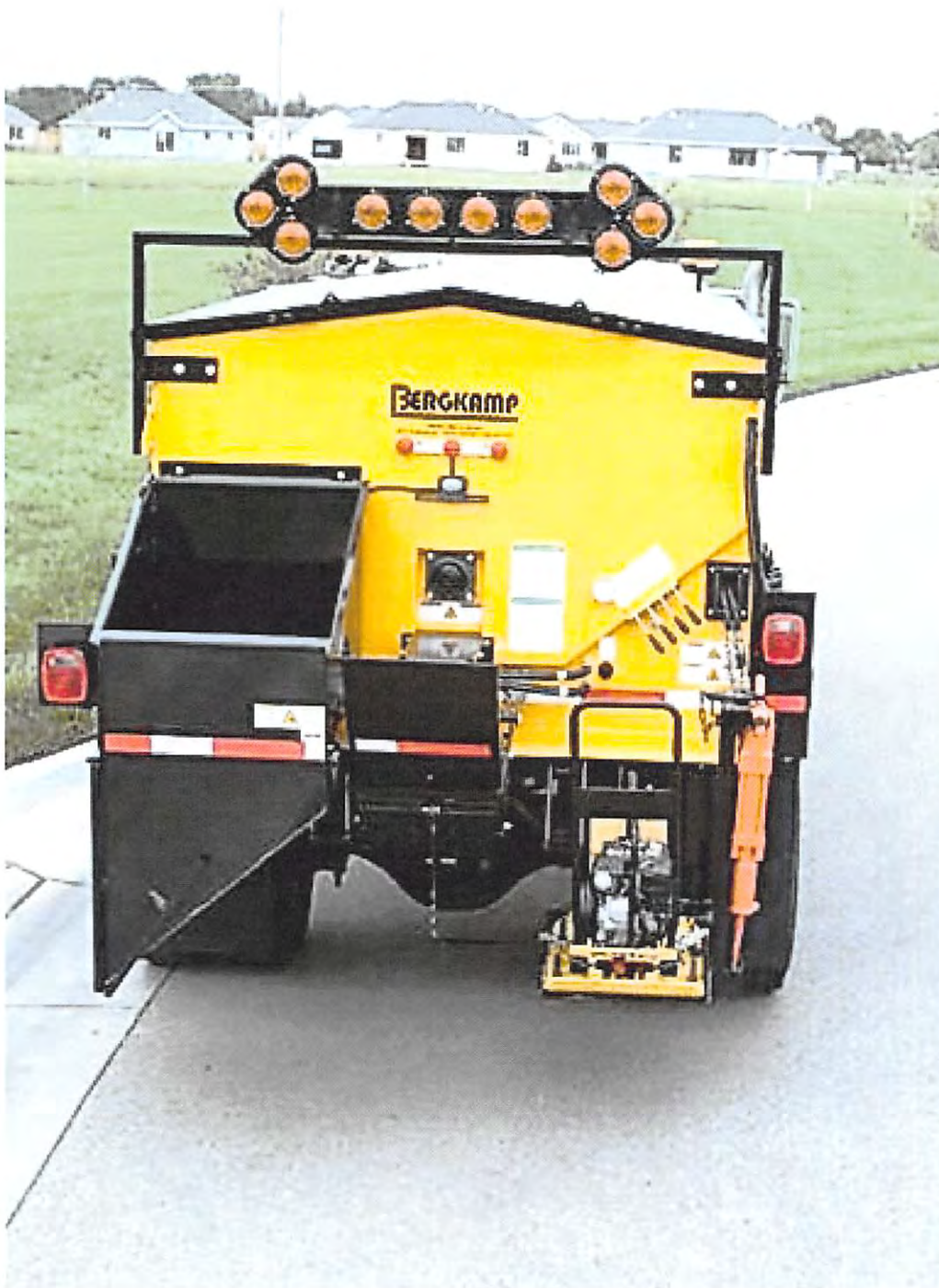
Shows hydraulic lift platform that houses Wacker Packer and pavement breaker
